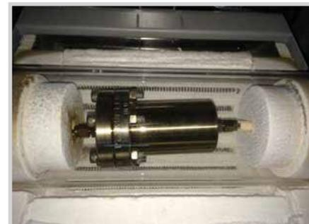
Fig 3: Thermal desorption unit and Sulfinert crucible used for thermal desorption testing of metal coupons
