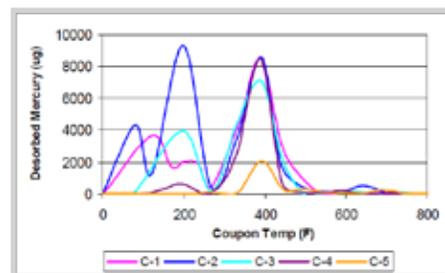
Fig 2: Thermal Desorption results of pre and post chemical treated mercury impacted metal coupons
